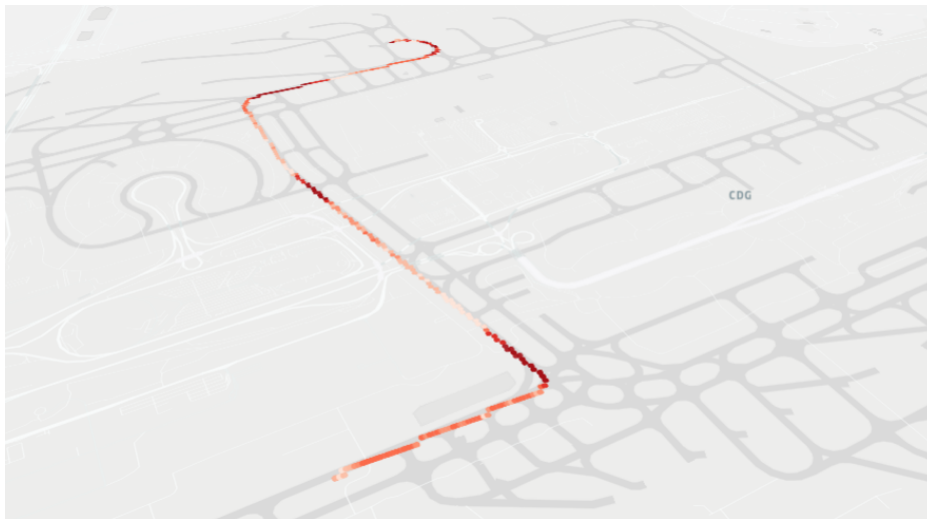
Figure 2.4: Considered trajectory (in red, the zones where the engine rate is high)
